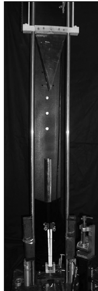
Fig. 2 The drop-tower setup in the Adhesion Science Laboratory.
